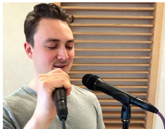
Figure 2. Two identical microphones 10-12 cm from the mouth of the subject. One microphone (mounted in a holder) is the reference, and the other is held in five different ways.
