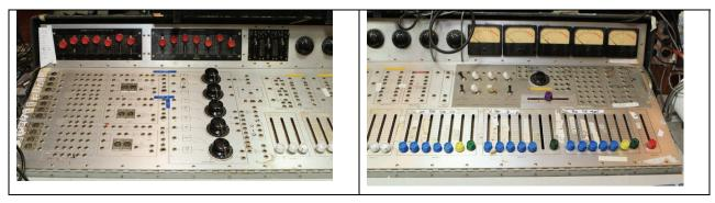
The faders are Langevins, as are the equalizers and rotary attenuators, and (of course) the 21 AM-16 amplifiers. Connections that would usually be wired/patched together are located next to each other, but they must be physically patched in order to be connected. EVERYTHING is 600-ohms input and output (sorta).
