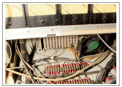
The thing with the waffle-grid heat sink is the power supply for the entire console.
