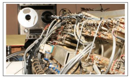
Mixer, looking from the left-hand side, to the right. At the bottom of the picture, is the harness going to the faders from the input patching.
