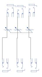
MASTER FADER NOTE: each output of the fader has 5 paralleled jacks
