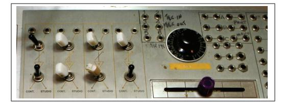
Under the VU meters, is the monitor switching. There are provisions for 4 monitors. If you look carefully, you can see the amplifier triangle pointing to the lower switch. In each monitor block, the upper switch selects the source, which is one of the two jacks, then there is a level control (the yellow knob) and then the power amp, and then the lower switch. The top switch typically did tape out vs tape in switching, and the bottom switch could select control room, both, or studio speakers.
